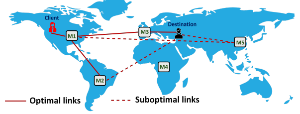
Figure 2: Latency optimization: A naive route selection leads to a suboptimal path like M_1 \rightarrow M_5 for a given destination, whereas DPR enables the selection of a highly optimal path such as M_1 \rightarrow M_3 .
